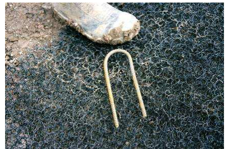
Typical U-shaped mild steel fixing pins
